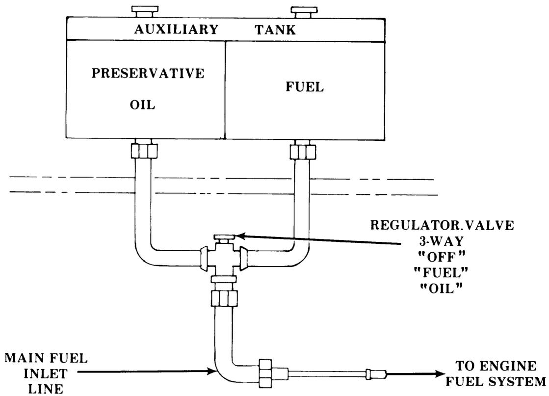
Figure 8. Auxiliary fuel container.
