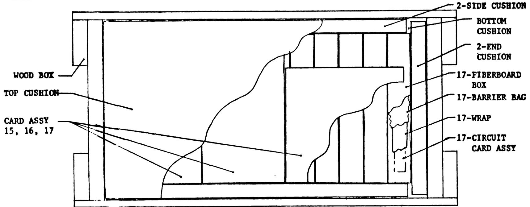
Figure 9. Packing configuration for printed circuit cards wood box.
