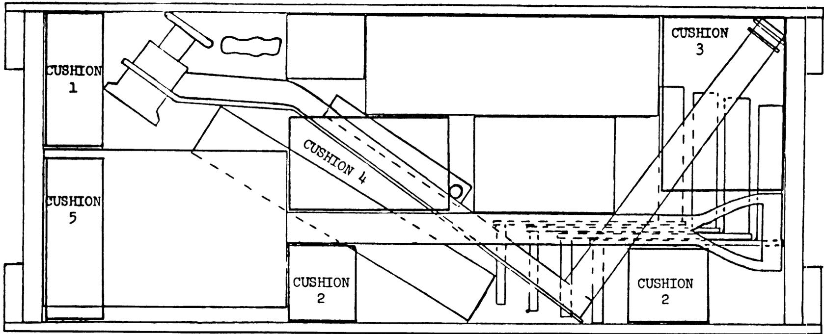
Figure 2. Packing configuration for OVE wood box.
