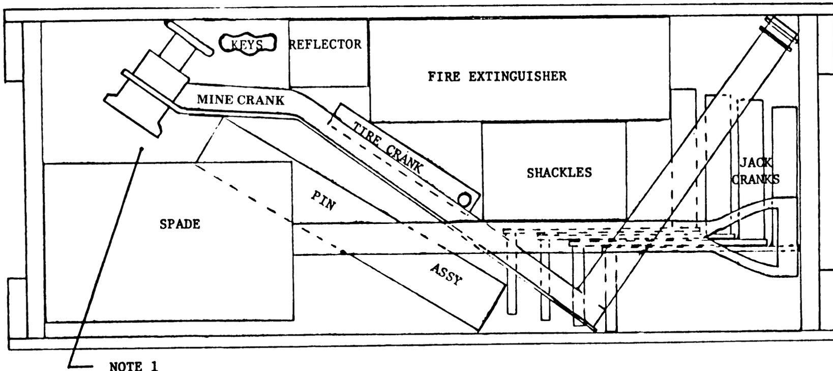
NOTE 1: Two belts in bag, packed in this area on top of spade and crank. Removed from figure for clarity.
